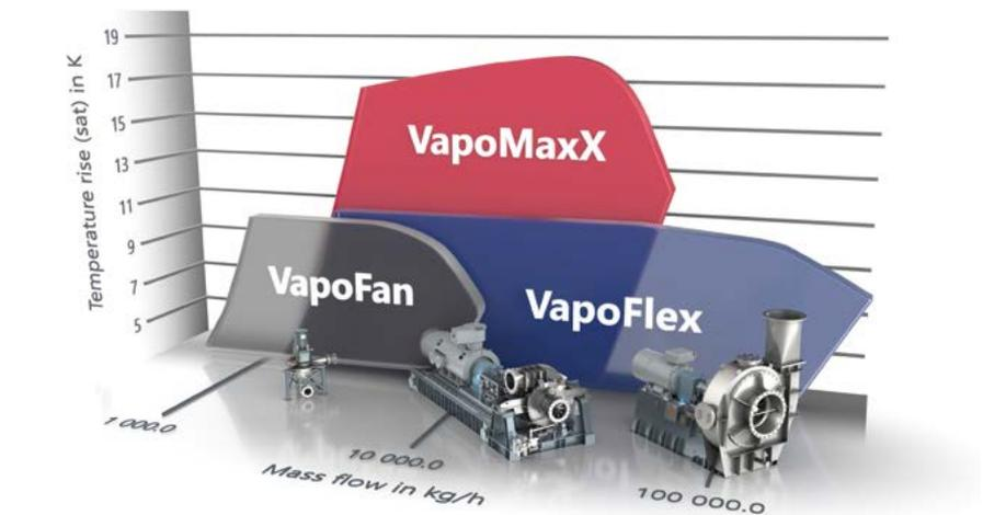
Performance ranges at 100 deg C inlet temperature
