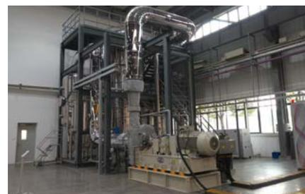
PILLER's falling-film evaporator in Taicang, China
