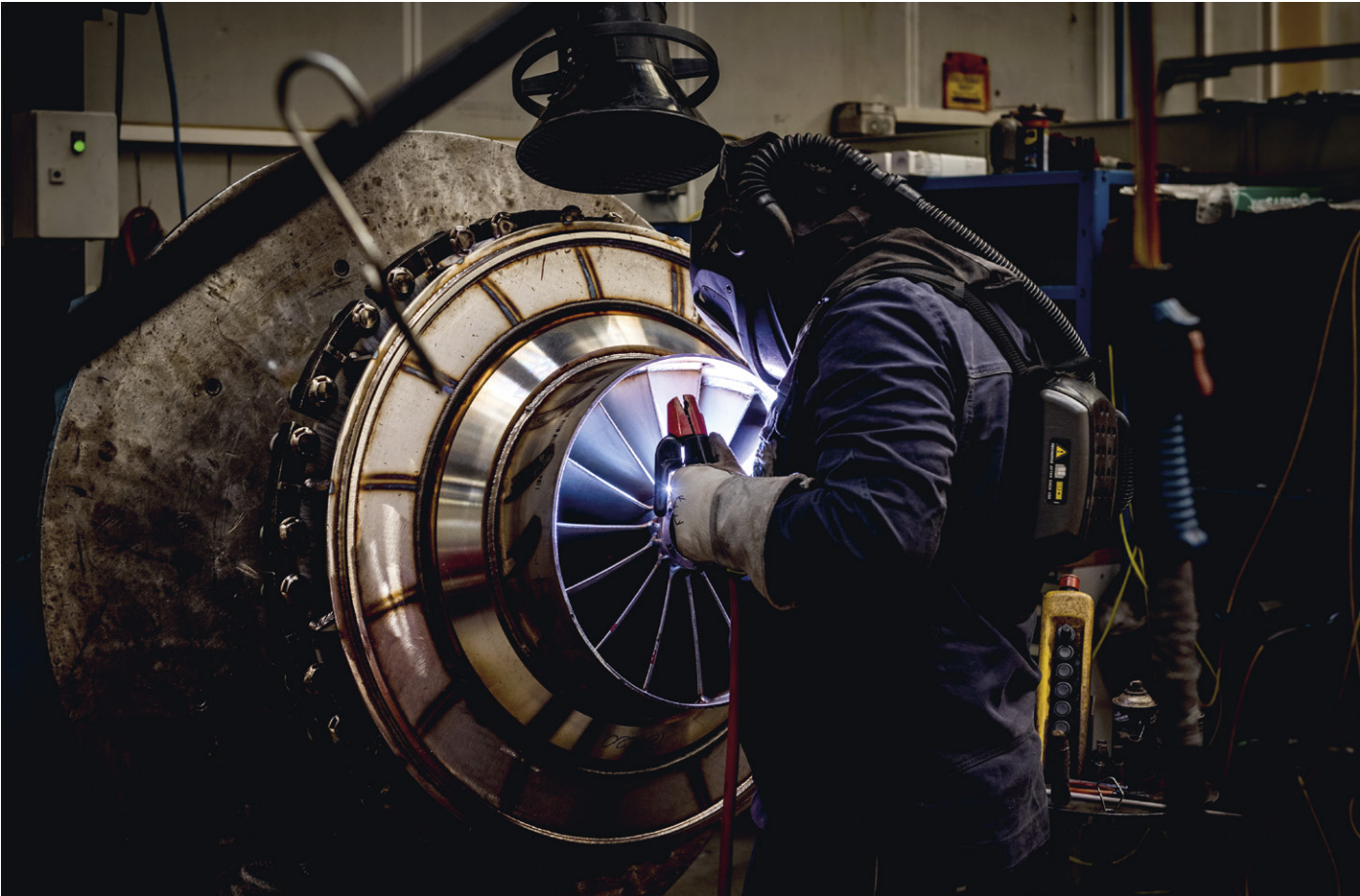
Craftsmanship: When welding the blowers, it is not possible in some hard-to-reach places without specialists with a sure touch.
