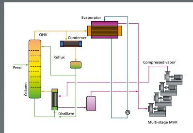
A schematic of an MSSR system with PILLER compressors integrated in one stripper and a MSSR system with four PILLER compressors for the second stripper. ROI achieved within just one year.
