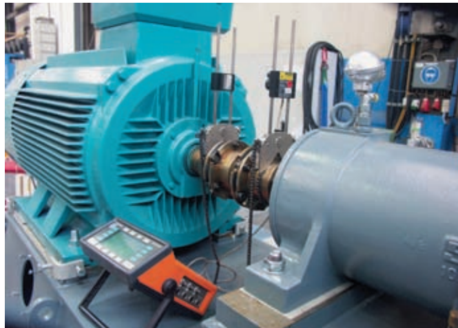
Precise alignment of coupling
