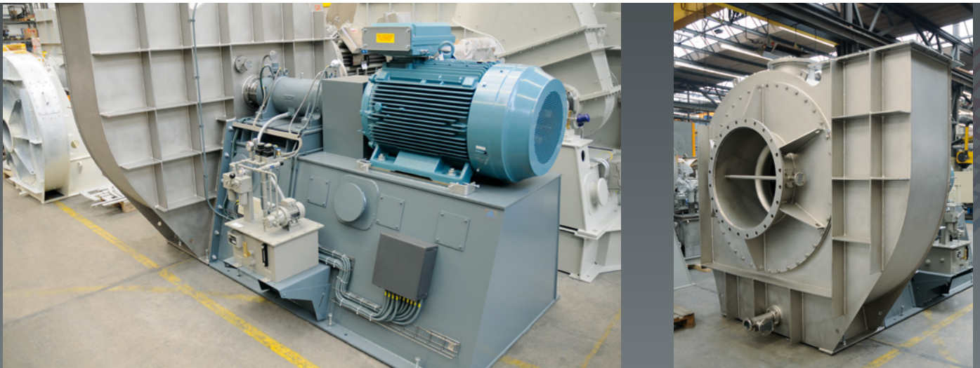
MVR Blower with Squeeze Oil Damper Bearing
